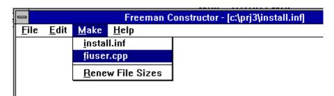
This will generate in c:\prj4 a file "fiuser.cpp" which is needed in the build.
